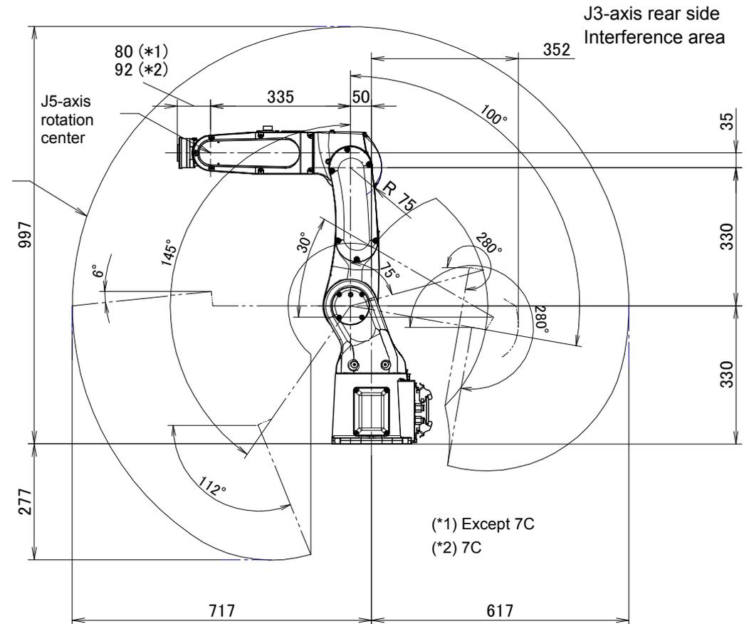
» If applied load on the robot exceeds 5kg when the robot is installed on an angle, the operating area is limited by the mount angle. If payload is less than 5kg, there is no restriction of the operating space.
